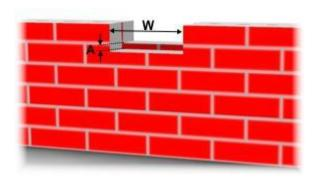
Leave the same gap of 260mm in the rear wall but extend it 20mm lower than the gap in the front wall.
