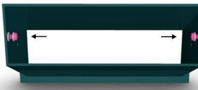
The rear chute has 2 sets of securing holes, the set required will depend on the depth of the wall. The diagram shows the set used for deeper walls. Place 2 nylon washers onto each of the 4 securing bolts and loosely screw into the securing holes. Position the washers as shown.
