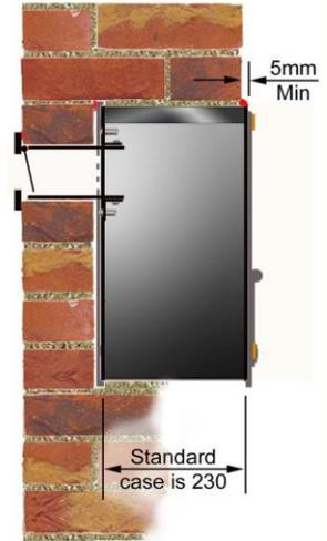
**Standard case shown fitted to thicker walls. Note deeper cases up to 900mm can be supplied**
